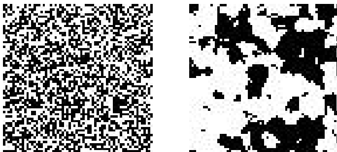
Fig. 6. Initial random image (left) and image after one iteration of the Partial Decoupling algorithm (right)
